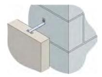
Tie fixed to blockwork restraining the top of a cast stone unit
