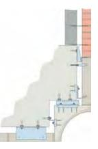
Support unit with special angles and channels for soffit and feature stones
