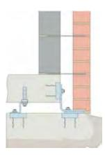
Continuous angle supporting brickwork above and cast stone units
