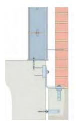
Continuous angle supporting brickwork above and cast stone units
