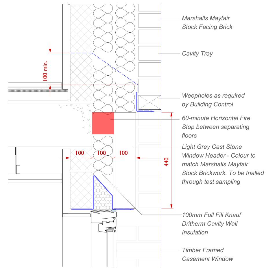
Cast Stone Window Header - Typical Detail Proposed - Scale 1:10 @ A3
