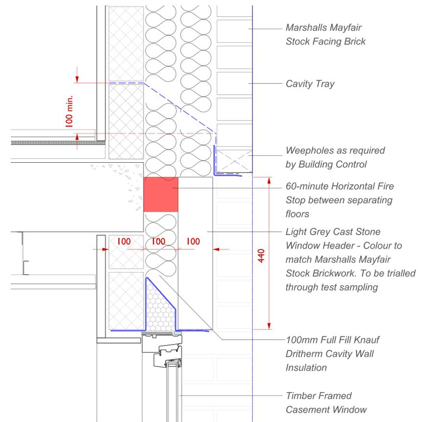
**Cast Stone Window Header - Typical Detail**
