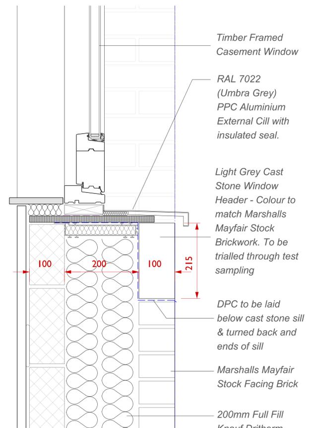
**Cast Stone Window Sill - Typical Detail**
