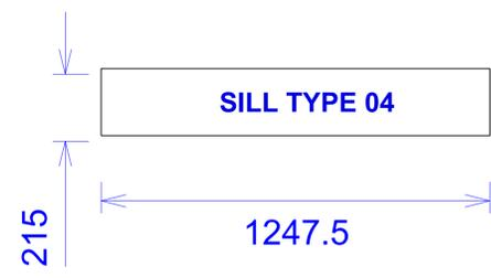
**Cast Stone Window Sill Types - Elevation**
